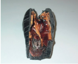
Fig. 6 – Data and visual evidence of a faulty motor connection
