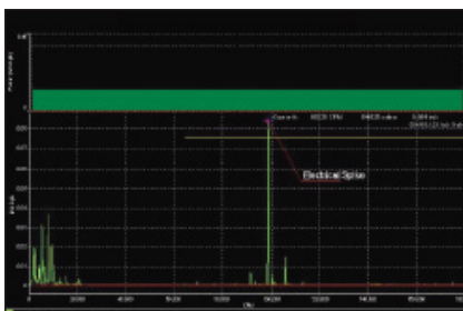
Fig. 3 – Vibration data showing an electrical defect (rotor issue)
