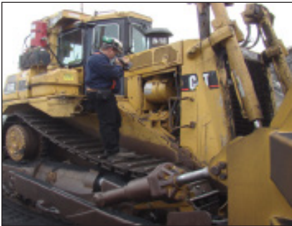
A Thermographer checks engine components such as exhaust ports, the turbo charger, accessory drives, fuel systems and heat exchangers.
