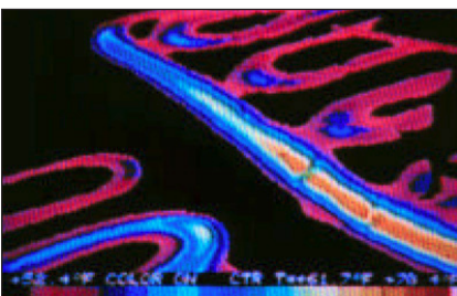
Image 8: Hydronic heating coils embedded in a concrete floor show up in this thermal image.
