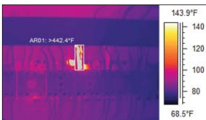
Figure 1. Example of Thermal Run-Away. Images taken over a 45 minute period during an inspection on May 22, 2003. The strands were arcing in the third image at 1:29 p.m. Images courtesy of Doug Gerhold.
