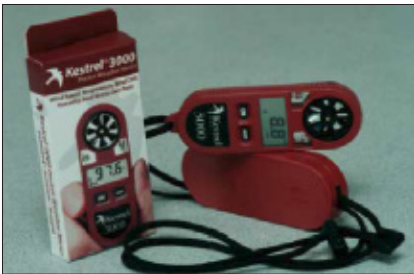
Figure 6. The Kestrel 3000 is an affordable solution to gathering accurate local climatic data essential to diagnosing IR problems.
